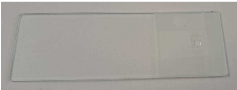
Figure 3.3: Typical PC-PDMS stamp used for stacking
