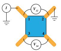
The figure above shows a four terminal, van der Pauw device made from a topological insulator. I is the applied current,  $V_{12} = V_1 - V_2$  the 2-probe voltage,  $V_{34} = V_3 - V_4$  the 4-probe voltage. As we explored in HW 11, the transport properties of a topological insulator can be explained in the Landauer-Büttiker (LB) formalism:
